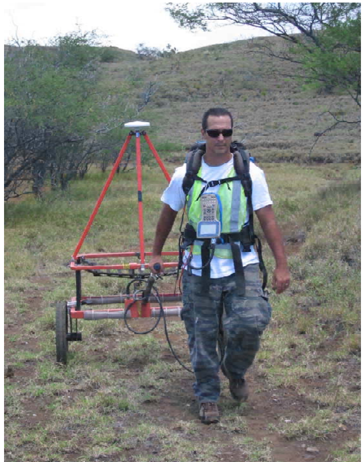
A certified technician uses a subsurface electromagnetic ordnance detector to locate unexploded ordnance at one Formerly Used Defense Site near Waikoloa Village on the Big Island of Hawaii. Crews have developed new methods which allow them to detect and clear 35 to 40 percent more land per day.
